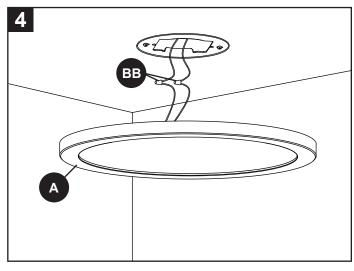
3.Use the wire connector (BB) to connect the N (nuetral wire) from the fixture to the N (nuetral wire) from the outlet box, connect the L (live wire) from the fixture to the L (live wire) from the outlet box.
